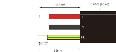
➤ Separate the AC plug into three parts as below.
