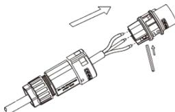
➤ Push the threaded sleeve into the socket, tighten up the cap on the terminal.
